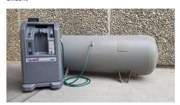
Oxygen concentrator uses PSA technology and makes oxygen from air. Now combined with the efficiency of gas mixing in nanobubble form, instead of air, increases the efficiency of aeration 500% and ozone production also.
